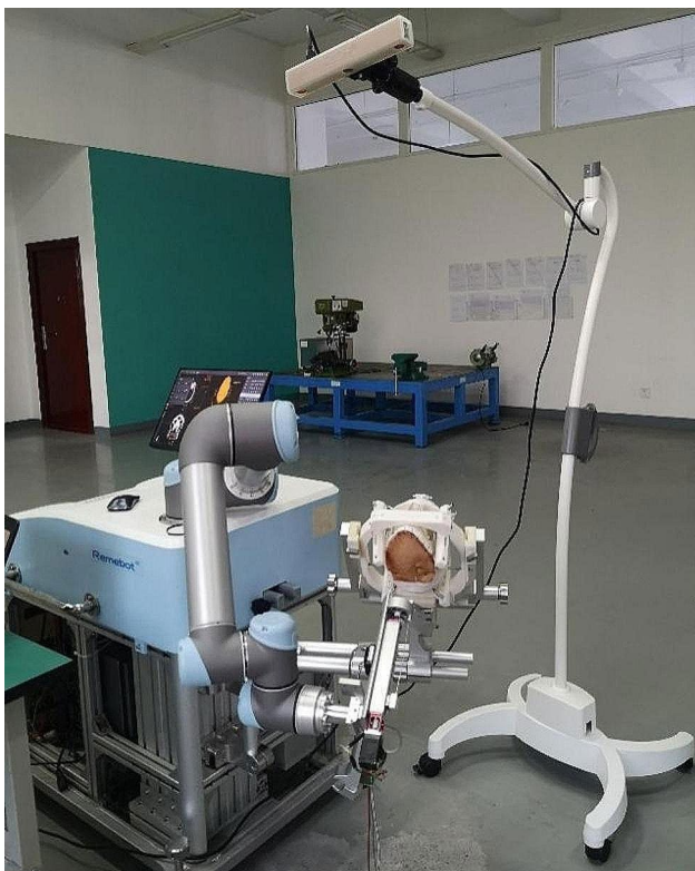
Fig. 1 Following the stabilization of the skull model's spatial position using a head frame, robot registration is performed
